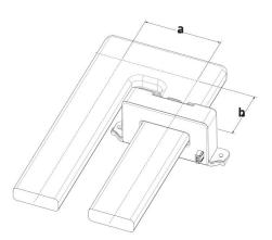
The qualification of the magnetic disturbances on the sensor is done using a U shape busbar.
